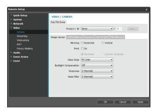
• **Pan/Tilt Driver**: Select the tab and configure the pan/ tilt driver. Specify the mounted pan/tilt driver's model and then set up an ID. Click **Port** and enter the pan/ tilt driver's port speed, data bit, stop bit, and parity values as per the driver manufacturer's instructions. DC-B1103 / DC-B1203 / DC-B1303 only
